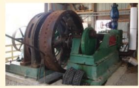
Running stationary Chuse steam engine from the handle factory in Hicksville, Ohio.
